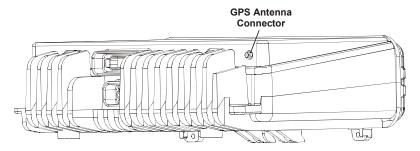
Figure 1. Location of GPS Antenna Connector on the MICOM
